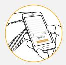
Tap the "Start measurement" button. A 15-second timer appears. You then have three seconds to position your smartphone's microphone as close as possible to the belt.
