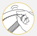
3 During the following 12 seconds, make the belt vibrate at the point specified by the vehicle manufacturer. You can do this by either flicking it hard on the side or hitting the back of the belt gently with a solid, blunt object (preferably made of metal)
